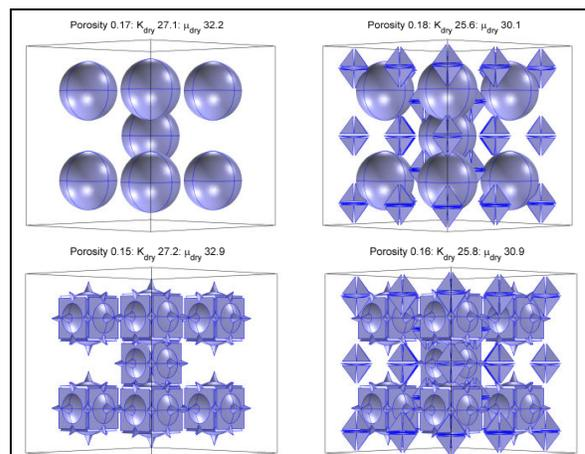
Figure 3: Four pore geometries for FEM calculations shown in Figure 4. Quartz frame is transparent.
