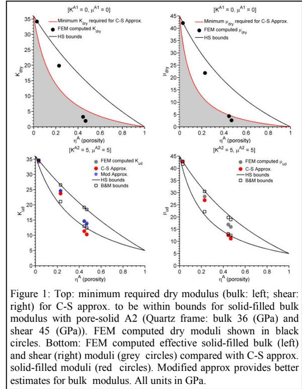
Figure 1: Top: minimum required dry modulus (bulk: left; shear: right) for C-S approx. to be within bounds for solid-filled bulk modulus with pore-solid A2 (Quartz frame: bulk 36 (GPa) and shear 45 (GPa)). FEM computed dry moduli shown in black circles. Bottom: FEM computed effective solid-filled bulk (left) and shear (right) moduli (grey circles) compared with C-S approx. solid-filled moduli (red circles). Modified approx provides better estimates for bulk modulus. All units in GPa.
