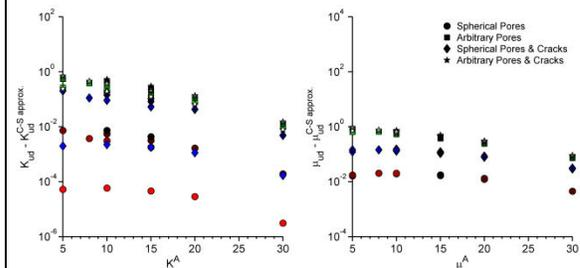
Figure 4: Difference between FEM computed solid-filled effective modulus and C-S approx. predicted modulus. Effective bulk (left) and shear (right) colorcoded with pore-filling solid's shear and bulk moduli, respectively. The colorcoded pore-filling shear modulus varies between 0 and 15 GPa for the effective bulk modulus plot and viceversa for effective shear modulus. Quartz frame and all units in GPa.
