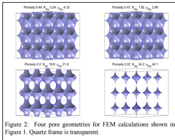
Figure 2: Four pore geometries for FEM calculations shown in Figure 1. Quartz frame is transparent.
